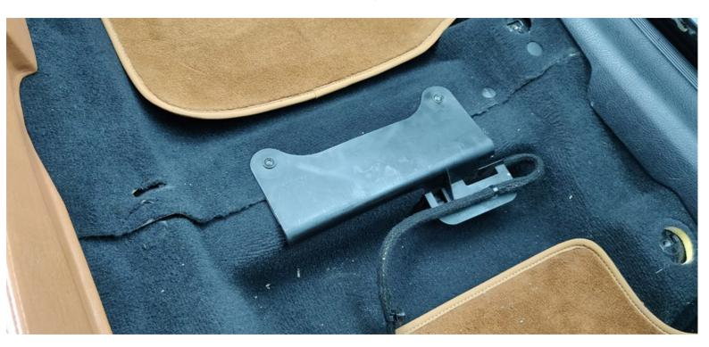
Underneath the seats are plastic covers, kept in place by some torx bolts (3 on driver's side, 2 on passenger's side). Remove these to get down to the carpet. Finally, disconnect the battery now to prevent any electrical issues from occurring.
