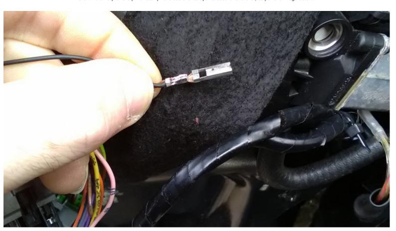
Moving on, we'll have to cut off a short piece of 'jumper' wire, and solder that to one of the pins. About 3-4 inches should be plenty here. Next, solder the remaining length of the new wire to the other pin. Lastly, solder the exposed end of the 'jumper' wire to the other pin. You should now have both pins connected through the jumper wire, and the rest of the new wire coming out of one of the pins. Now:
