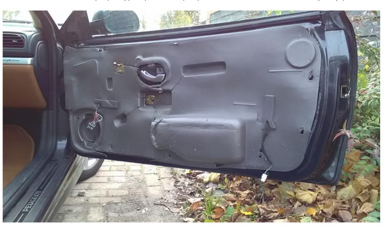
Next, disconnect and remove the speaker. Four Philips screws keep it in place. Now you should be able to take off the grey insulation layer. If this has never been done in your car, you might have to cut along some parts that sandwich the material between part and door. Hopefully, yours doesn't look as gutted as mine. The inside of the door should now be visible, which looks like this:
