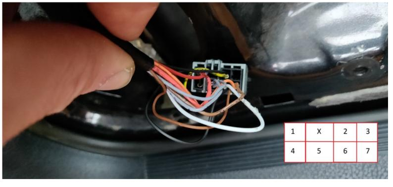
Looking at the window switch's connector FROM THE BACK, I've numbered the pins as follows (see picture). Note the X in my diagram; this is where the securing pin of the connector is. On the driver's side, you can already see quite clearly the differences between the automatic and manual connectors. Here, we'll be rearranging some of the pins already present, we'll cut some others, and make some new connections. Let's do it:
