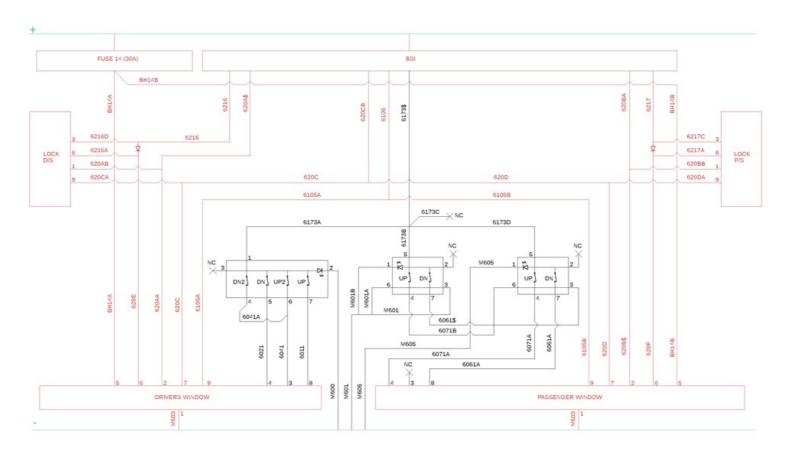
Note: Some of the wiring in this second diagram have no identification. These will be the wires we have to add ourselves.
