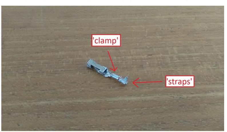
Take out your soldering station and new wire. Before doing anything, consider how you'd like to make the new connection. In my experience, the best way is to solder the wire on top of the pin's 'clamp' and use the 'straps' to secure it further, as per the image below:
