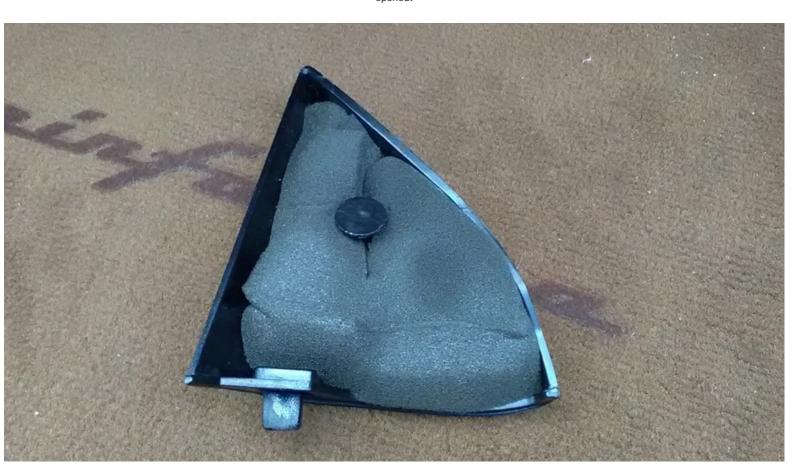
The rest of the door card is kept in place by plastic pins that can be pried/pulled off. It's best to start on the bottom and work your way upward.
