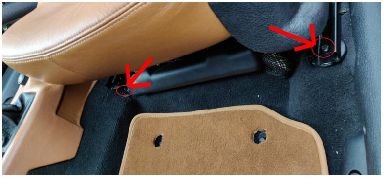
Next, we'll remove the seats: Four bolts keep them in place. Start off by moving the seat forward, and remove the rear bolts. Now move the seat backward and remove them from the car.
