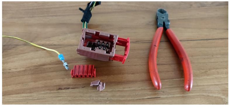
First, we'll prepare the pin we're going to insert into the window mechanism connector. Since we can simply push this in from the rear, the spare connector may be harmed in the process. I simply cut up the plastic surrounding the pins, as to extract the pin in perfect condition. Note the blue rubber part connected to the pin. Leave this, and a part of the wire connected, as it'll serve as a gasket for any water that enters the inside of your door.
